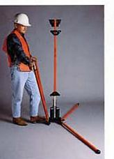
3. Walk to the other side of the Little Buster stand, place your left foot on both release levers and step down. The remaining two legs will fall to the ground.
