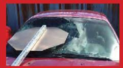
No Breakaway Device = High risk of occupant injury. At impact, the sign post can be forced into the windshield and roof of the vehicle.
